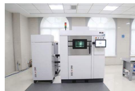
EOS M290植入物3D打印 EOS M290 Selective Laser Melting (SLS) Equipment
